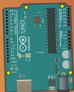
COLLEGANDO ARDUINO A UN COMPUTER CON UN CAVO USB FORNIAMO L'ALIMENTAZIONE E POSSIAMO COMINCIARE A PROGRAMMARLO.
